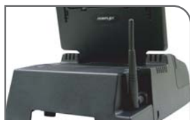
Optional WLAN module supports IEEE 802.11 a/b/g and WinCE driver.
