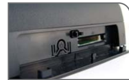
CF card slot for optional CF memory card which allows booting from HDD or optional CFcard.
